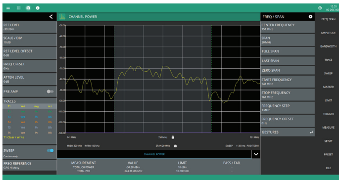
Common Spectrum Analyzer Measurements Including Channel Power are Automated with Smart Measurements
